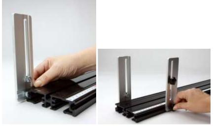
2. Mount the Photogate or Distance sensor on the bracket using the star-knobbed bolt provided.
